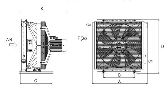
Max static pressure: 21 bar Max Dynamic pressure: 14 bar\*\*
